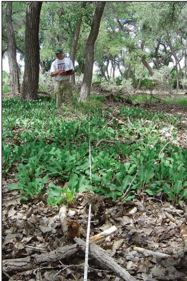
Figure 3-12. A tape measure laid out to measure vegetation using the line intercept method, a transect-based method.
