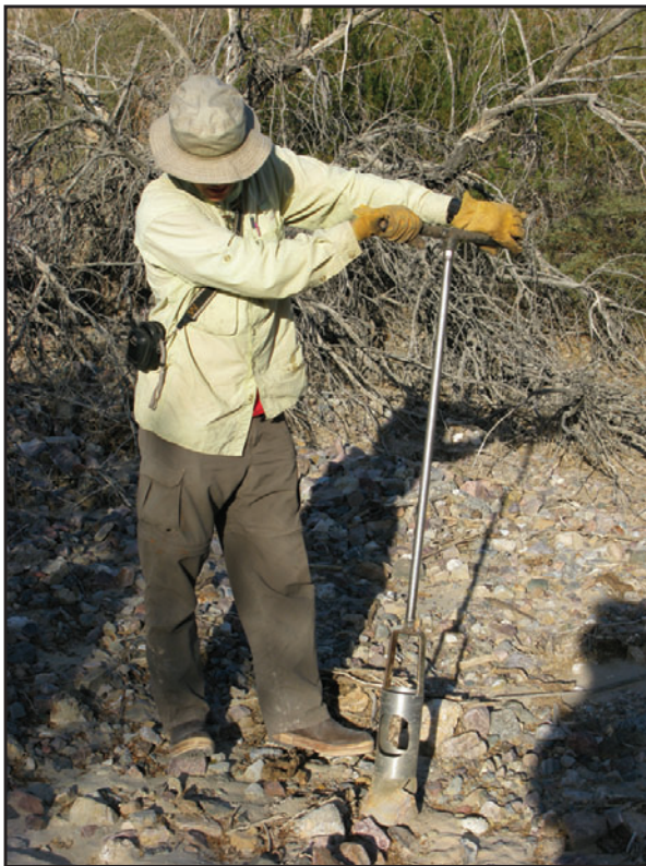
Figure 4-5. Hand augers can be used to bore holes for installing a groundwater monitoring well. Mounted power augers may be used in cobble or hardpan substrate.
