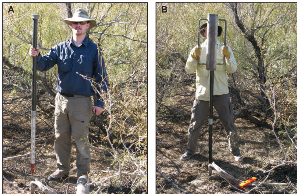
Figure 4-8. Steel drive points can be pounded into the ground to create water table monitoring wells or piezometers.
