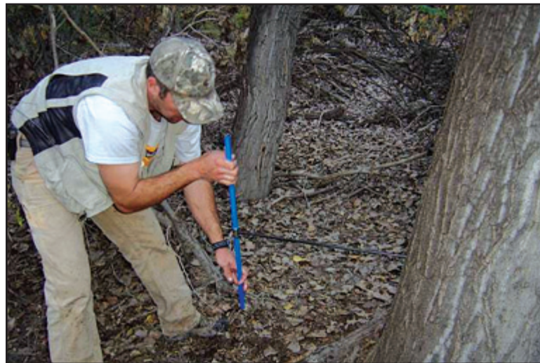
Figure 3-10. An increment borer may be used to collect cores of trees and shrubs. Cores are then dried, mounted onto a board, sanded, and polished. Rings are counted or ring widths are measured to determine age or growth rate, respectively.
