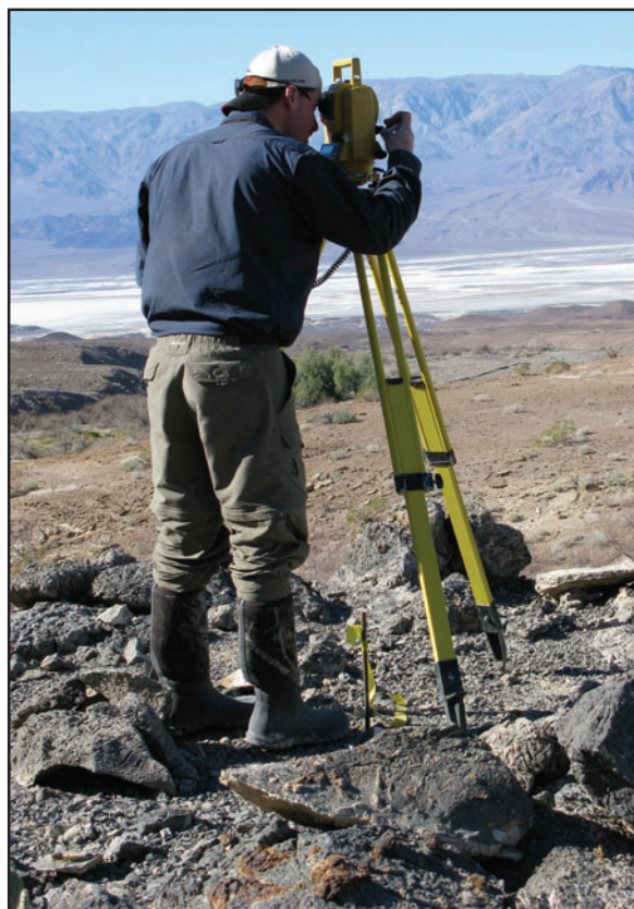
Figure 4-18. Topographic surveying with full station in Death Valley National Park, California.
