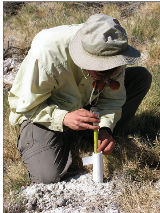
Figure 4-9. Manual measure of water table depth in monitoring well using a tape measure.
