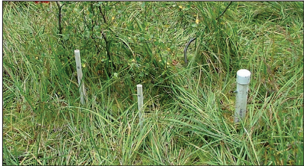
Figure 4-7. A well nest consisting of one water table well (right) and two piezometers.
