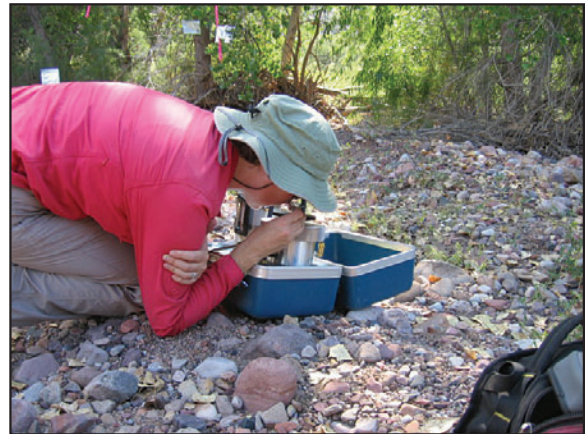
Figure 3-5. Left: cross section of pressure bomb showing cut leaf (or twig) inside the chamber with the cut end protruding through the rubber stopper and chamber top. The exhaust valve is closed and pressure increased until water flows back through the xylem and is expressed on the cut leaf or twig surface (top right). The researcher carefully watches the cut surface as the pressure increases, recording the pressure at which the water emerges (bottom right).
