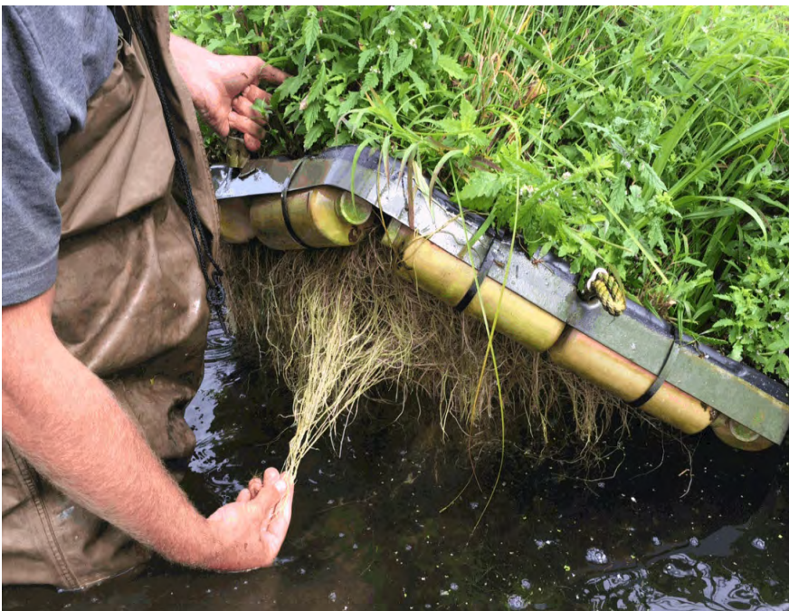
FIGURE 16. PhytoLinks module showing HDPE-encased flotation system.
