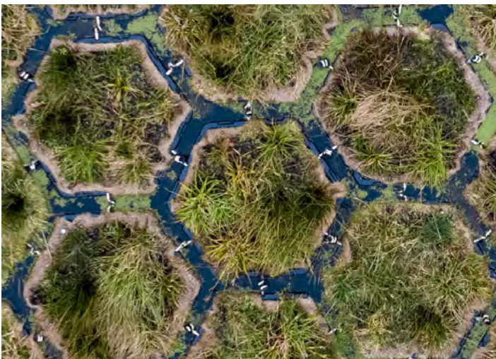
FIGURE 13. Mature PhytoLinks modules showing module-module tethering and quick attach connections.
